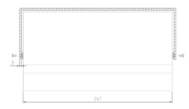
The bracket is fixed on the ceiling or wall by screws. This installing is possible due to the bracket contains drills in its bigger wing.
